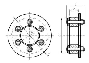
WA-GPPLR pipe seals has one of the plate rings enlarged for anchoring the seal against hammer shock.
