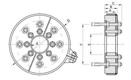
External Wall Mount Pipe Seals WA-GPB waterproof a pipe penetration from outside the wall. It can mount on an inner or outer wall.. The units are a low profile 2 3/4" thick, that may be installed in a restricted space area. Where mounting space is less restricted a <u>WA-GPT external wall seal</u> assembly is more suitable.
