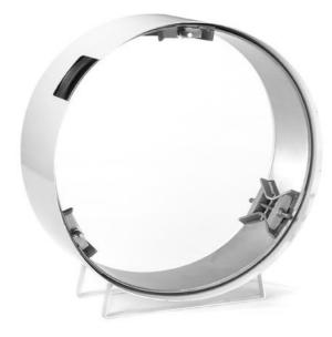
Internal repair clamps can be installed inside pipes of various materials. Fit sizing from 20 inch / 500 mm - or larger. Operating pressure can be up to 240 psi / 16 bar.
